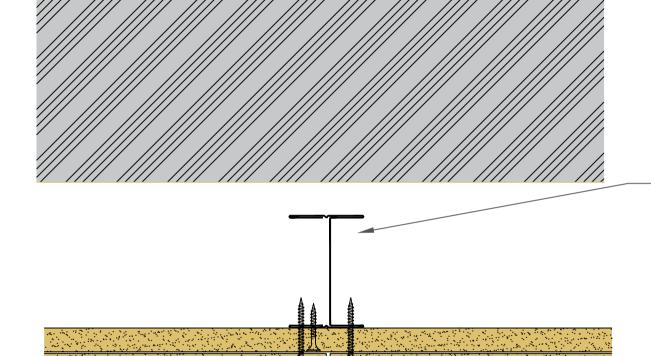
SPEEDLINE 60mm 'I' Studs at 600mm Ctrs
